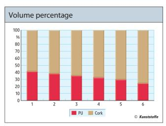
Fig. 5. The limiting range (No. 6) is achieved at a mixing ratio of 75 vol.-% cork and 25 vol.-% PU
