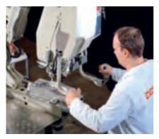
Fig. 11. The manually guided casting head ensures high flexibility during production
