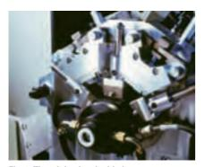
Fig. 2. The mixing head with three component valves and positive synchronisation permits high quality without premature advance of one component
