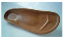
Fig. 8. Example of a cork/PU shoe sole with a proportion of 15 wt.-% cork
