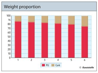
Fig. 4. The limiting range (No. 6) is achieved at a mixing ratio of 25 wt.-% cork and 75 wt.-% PU
