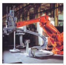
Fig. 12. The robot-guided mixing head operates flexibly and with high productivity
