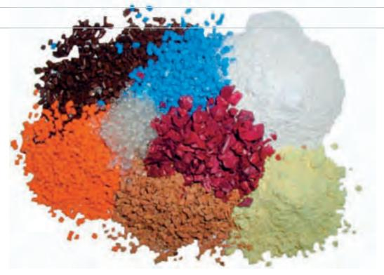
Regrind of cork, calcium carbonate, rubber, TPU and physical blowing agents (photos: Desma)
