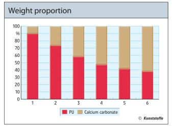
Fig. 6. The limiting range (No. 6) is achieved at a mixing ratio of 61 wt.-% calcium carbonate and 39 wt.-%  $\rm PU$
