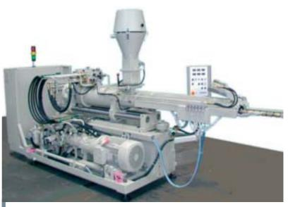
Fig. 3: Thermoplastic injection unit
