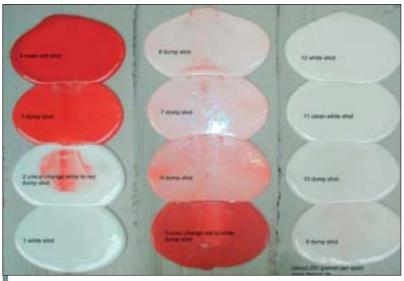
Fig. 1: Example of a colour change-over with Desma technology
