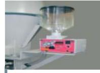
Fig. 5: Addition of dry colorant according to the masterbatch method
